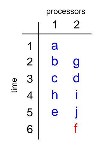
Work = 10, Span = 5, so Brent's Theorem suggests  $5 = \max(10/2, 5)$  time steps might be possible. But we have some idle times, so get 6. (Also: Brent's Theorem is only an asymptotic assertion.)
