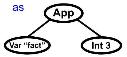
A parser produces ASTs. A typechecker and evaluator can then traverse them.
